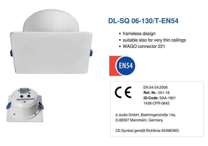
Inspired by the look of contemporary LED lights, the frameless design of the new 6W loudspeakers has all the makings of an instant classic. The 6W powered square speaker is equipped with a 130mm full-range loudspeaker and a 100V transformer with 3 power adjustments. The powder coated metal in RAL 9016 guarantees long-term stability. For additional reliability the speaker is impregnated against wetness.
